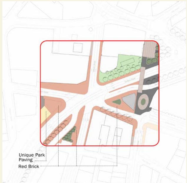
Recommendation Option 3: Same as Option 2, but carry red brick paving to threshold gate at egress stair structure. Also make changes to Dewey Square design by replacing grey brick with red brick west of the vent structure at Essex Street. This change will require modifications to C17A6 that will necessitate an additional funding source
