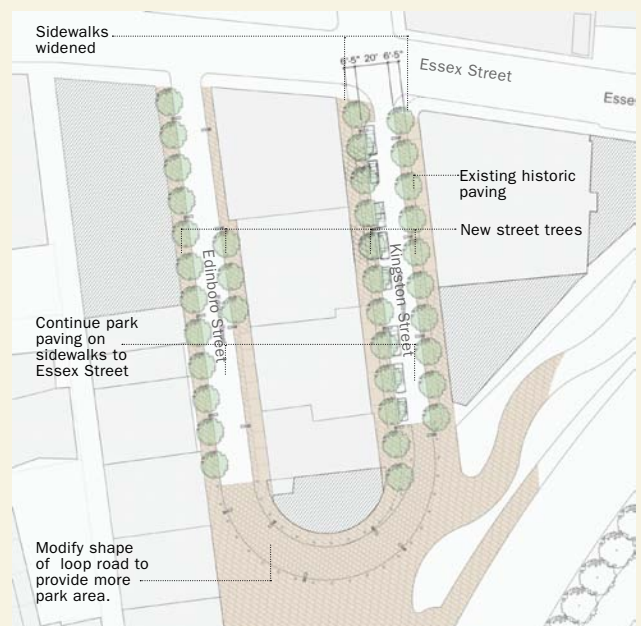
Recommendation Option 3: Widen sidewalks to allow for street trees. Extend park paving along sidewalks and "loop". Modify "loop" configuration
